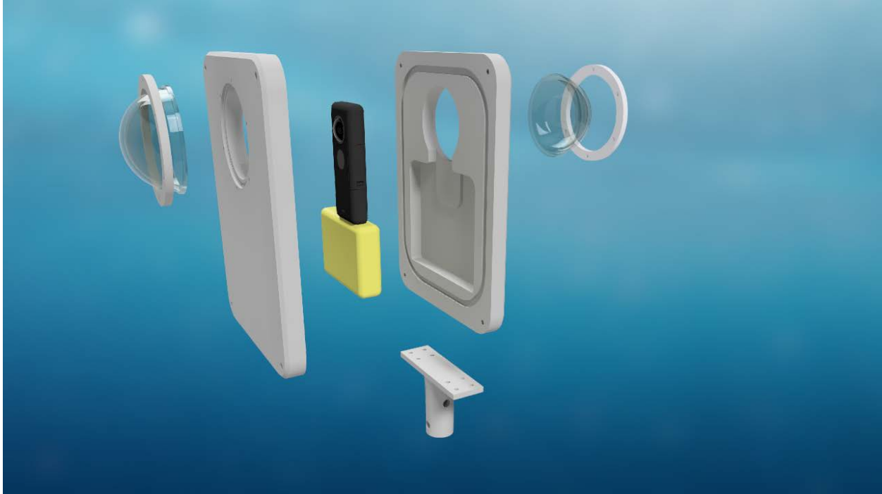
Figure 5 Insta 360 One X Pressure Housing Design.
