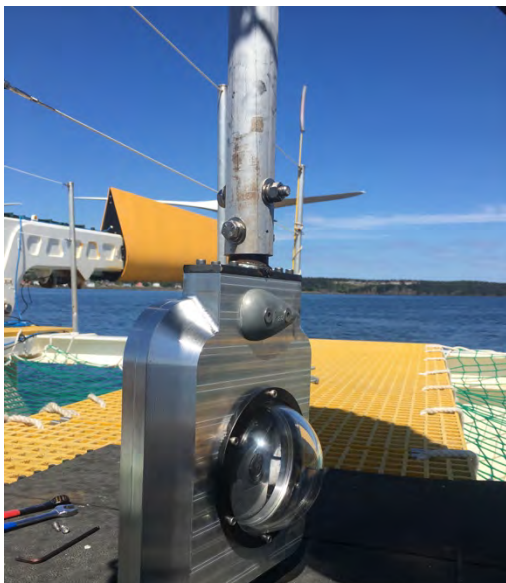
Figure 2 Go Pro Fusion System Attached to Scaffolding Pole in Preparation to be Mounted to the PLAT-I.
