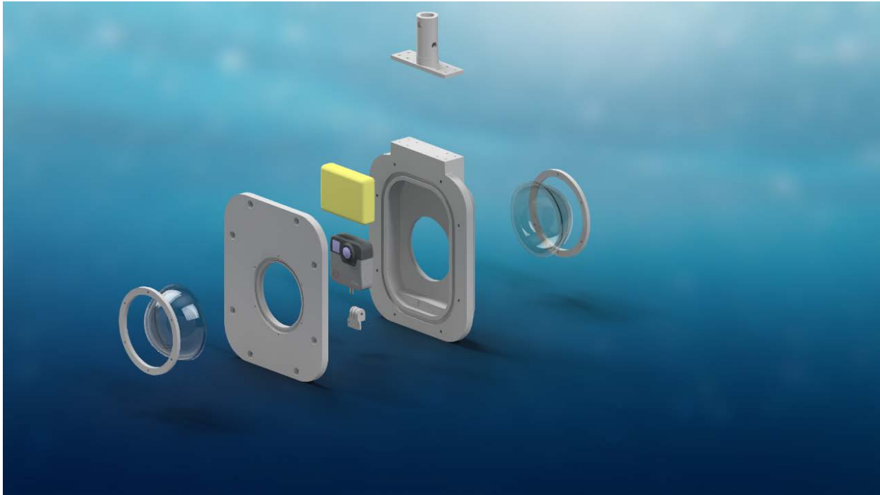
Figure 4 Go Pro Fusion Pressure Housing Design.
